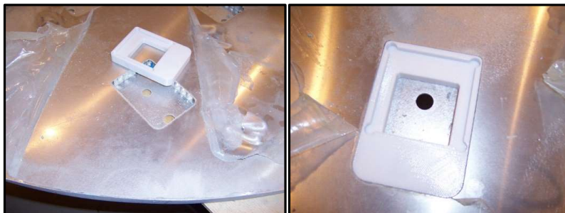
Figure 10. Close-up of central plate construction. Left – Machined aluminum cutout and holder, Right – Assembled unit [Source: NASA]
