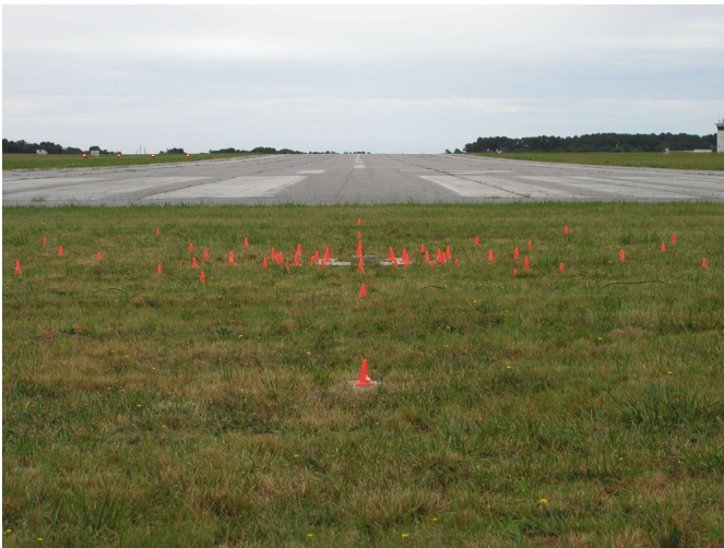
Figure 1. Overrun Area of WFF Runway 17, showing covered array microphones. [Source: NASA]
