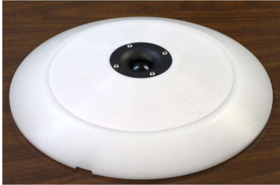
Figure 43. Tweeter mounted on ground plate. [Source: NASA]
