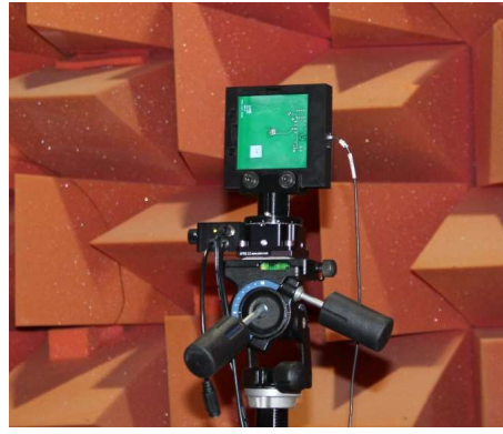
Figure 23. Microphone casing for directivity measurements.
