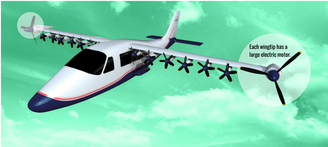
Figure 5. Concept Image of Mod IV, the X-57 Maxwell Airplane with Cruise Propellers and High-Lift Propellers Operating [Source: NASA / Advanced Concepts Lab].
