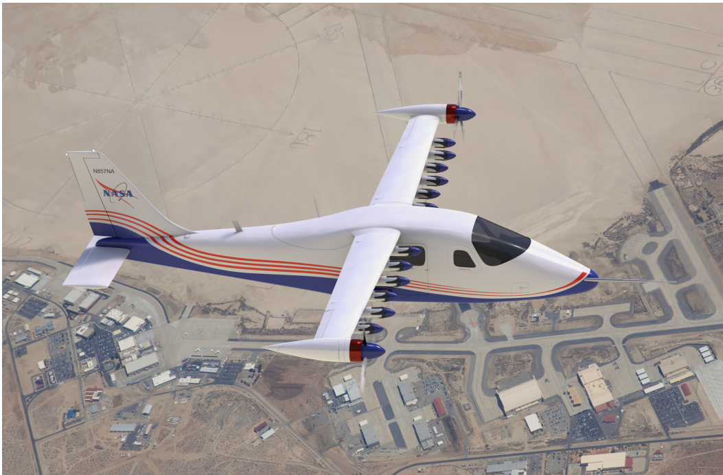
Figure 4. Concept Image of Mod III, the X-57 Maxwell Airplane with Cruise Propellers Operating and High-Lift Propellers Stowed [Source: NASA / Advanced Concepts Lab].
