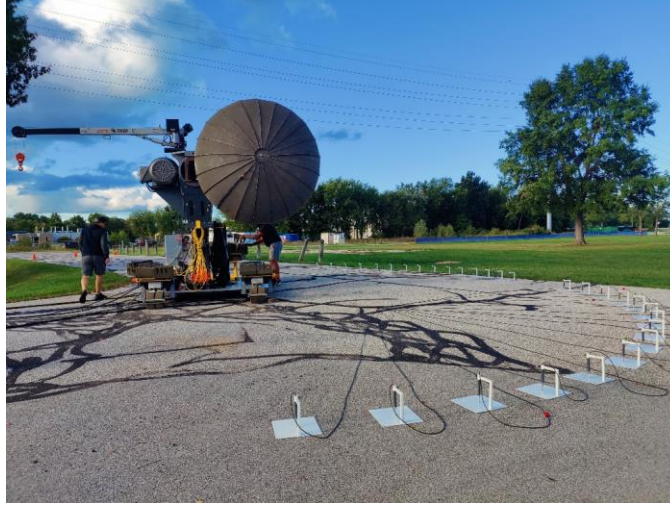
Fig. 9 ANCF test setup to acquire far field data for baseline and liner configurations
