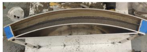
Partially filled Materials separated by the steel grid
