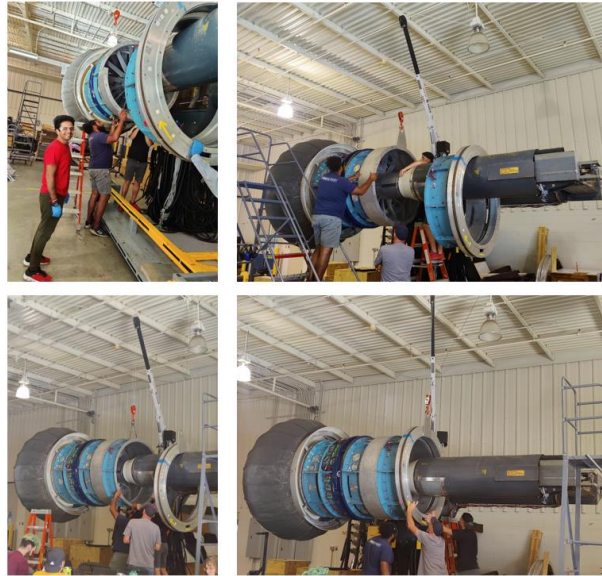
Fig. 7 Liner installed holder assembly into ANCF test rig
