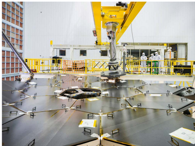
Figure 11. Installation of the final Primary Mirror segment, assisted by a high-precision robotic arm, suspended from traveling stages. Black covers were mounted on the mirrors to protect from contamination.
