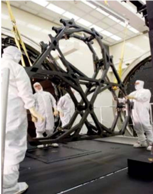
Figure 8. The Backplane Stability Test Article (BSTA) was an engineering model for 1/6 of the JWST backplane, including the structural elements used to create the entire backplane assembly. This shows the BSTA being prepared for cryotesting at operational temperatures in the XRCF.
