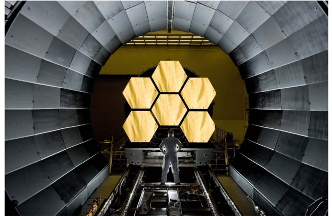
Figure 7. Six of the flight mirror segments prepared to undergo acceptance testing in the XRCF. The segment-level optical performance and structural stability was precisely measured.
