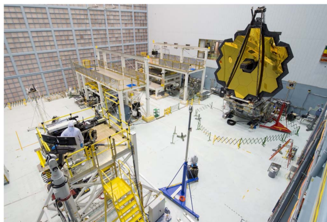
Figure 12. Center of Curvature test setup for ambient optical measurements of the PM. The high-speed interferometer, null lens, and CGH are mounted on the stable platform at lower left.
