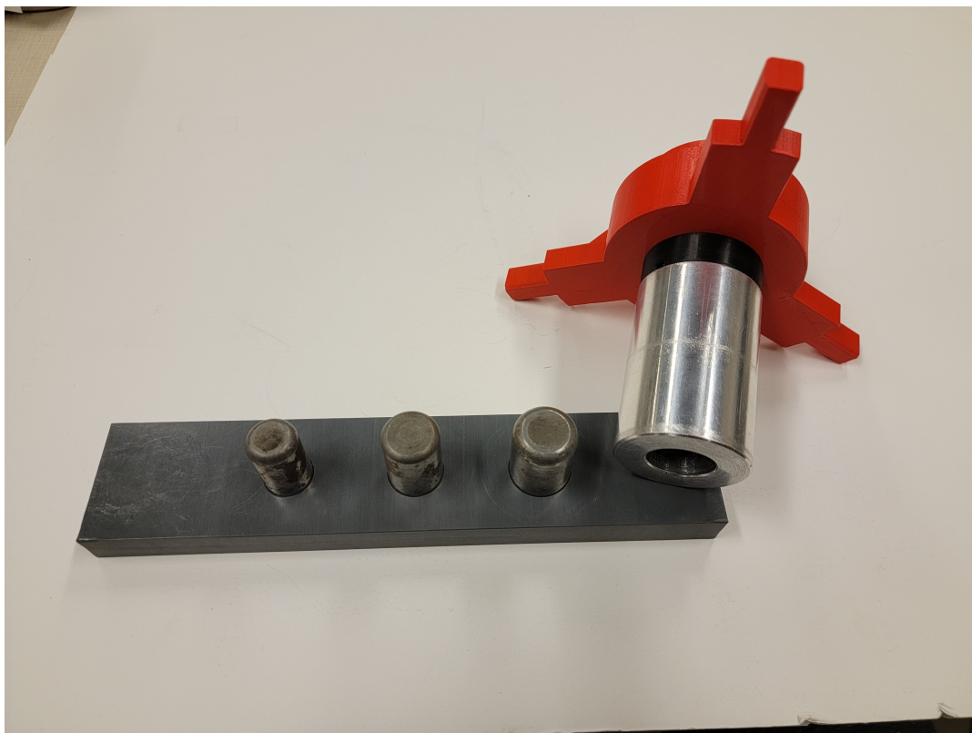
Figure 7. The Peg board with pegs from diameter of 0.5”, 0.75”, 1” next to the tool attached with the sleeve outer diameter of 2” and an inner diameter of 1.0035”. More info at Pokharna (2021b)
