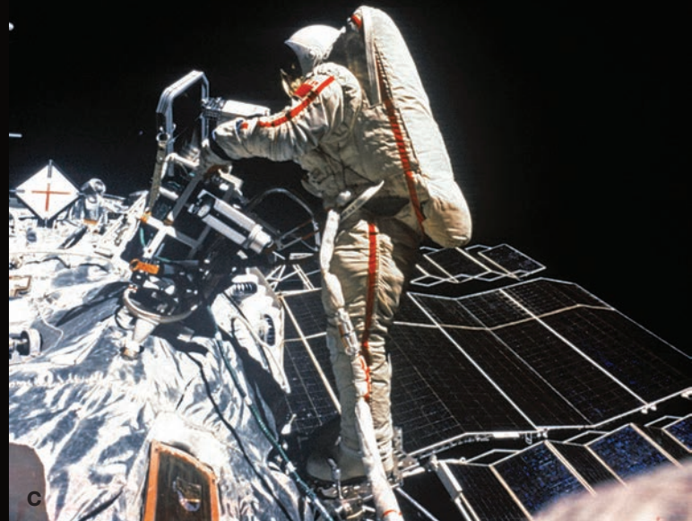
Fig. 1 — Space welding milestones. A — 1969, Soyuz 6 capsule using the Vulkan unit, representing the first space welds with electron beam, plasma arc, and gas metal arc welding (USSR); B — 1973, Skylab, experiment M551 with electron beam welding and experiment M552 with braze experiments (United States); C — 1984, Salyut 7, signifying the first manual open space welds (USSR). (Credits: NASA and O. Strelko.)
