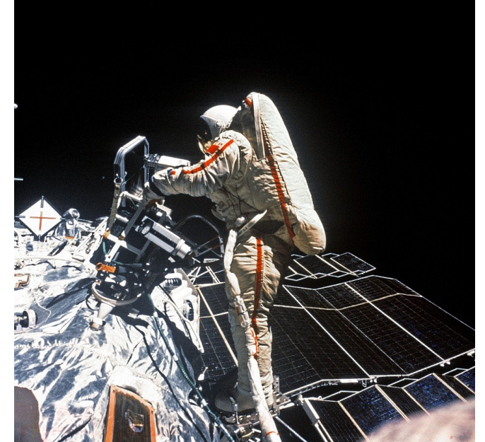
In Space Welding
