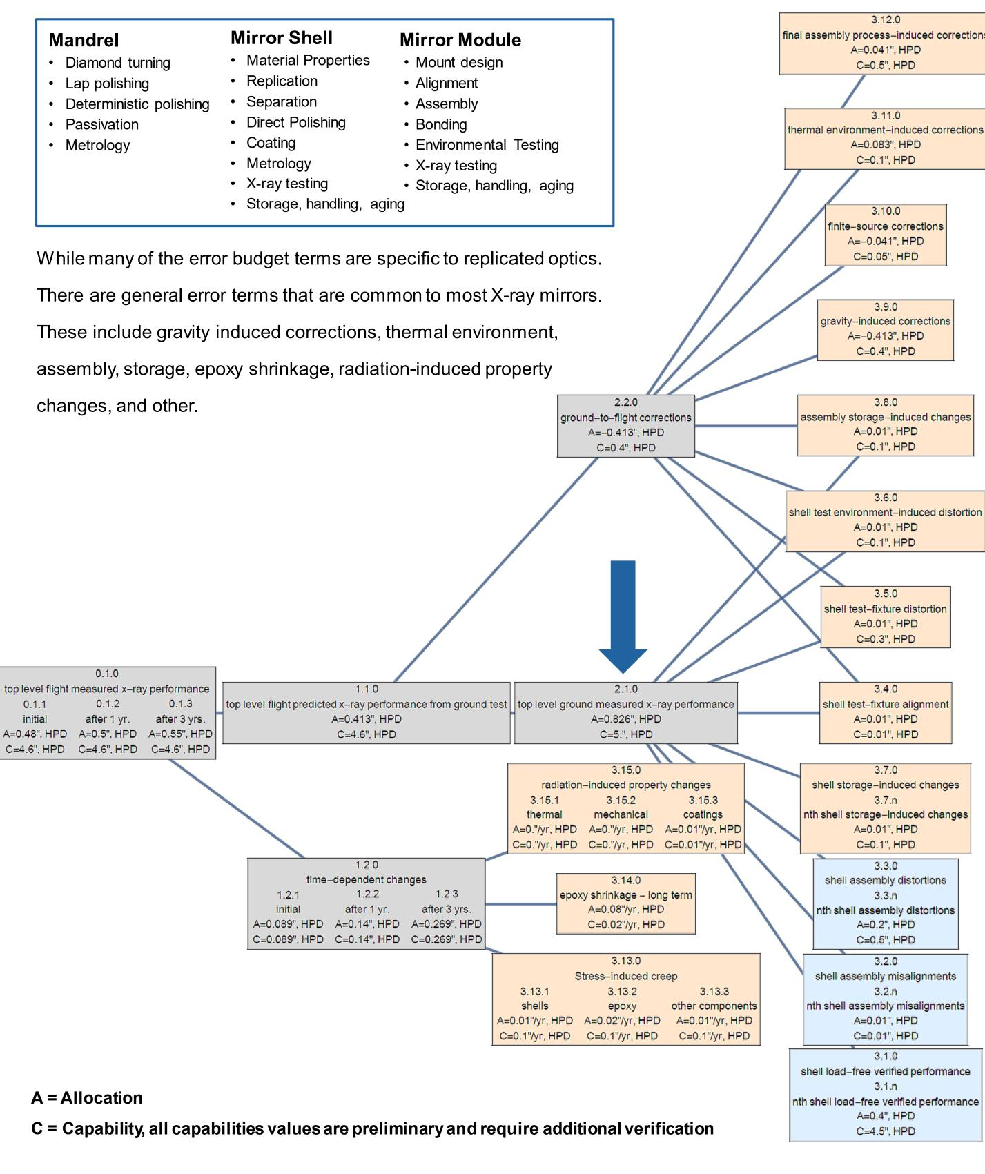
Gray Boxes = Post-Assembly (testing and aging) Blue Boxes = Individual Mirror Shells and Assembly (fabrication, assembly, and metrology) **Orange Boxes = Generic Terms (common to all X-ray mirrors and assemblies)**
