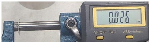
Free-standing LPSC Thin Films (~26 \mu\text{m} thickness)
