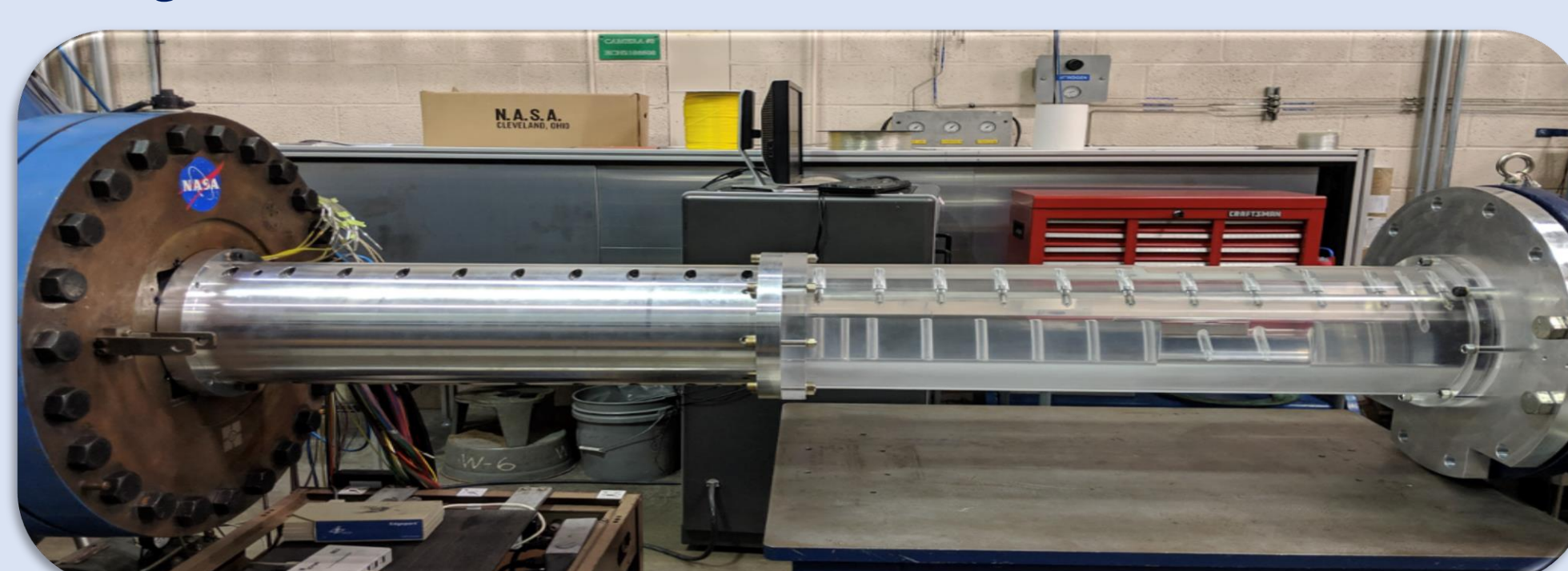
Supersonic tunnel at NASA Glenn with octagonal test-section
