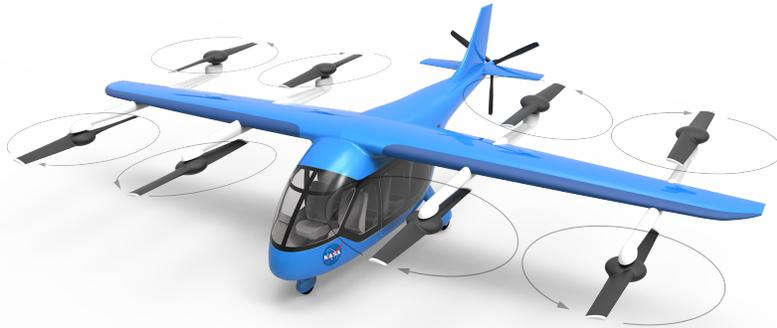
Figure 1: Rendering of the six-passenger Lift+Cruise reference aircraft.
