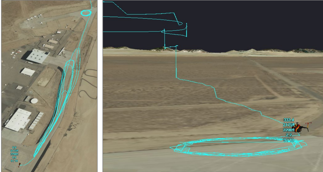
Figure 2.40. ADS-B SBSM track for pirouette and approach maneuvers.
