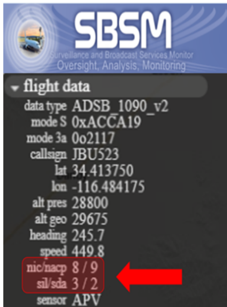
Figure 4.64. ADS-B Out, SIL and SDA with SBSM Example Flight Output.
