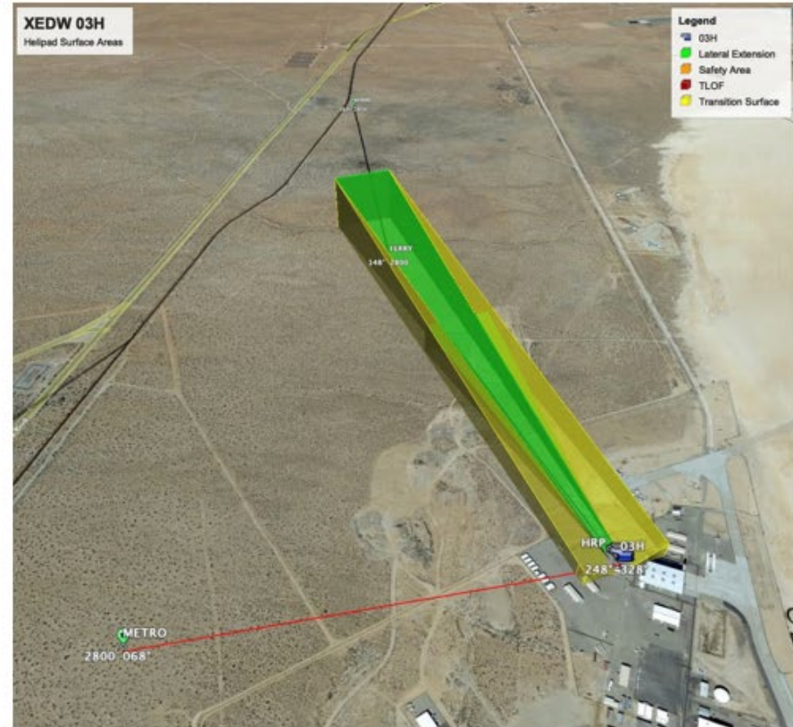
Depicts XEDW 03H selected for dynamic interface. the calculated magnetic variation, publication date, lat/long geodetic datum, and ellipsoidal heights in feet, surveyed thresholds required by the FAA to be accurate in any landing surface with a takeoff or approach procedure.
