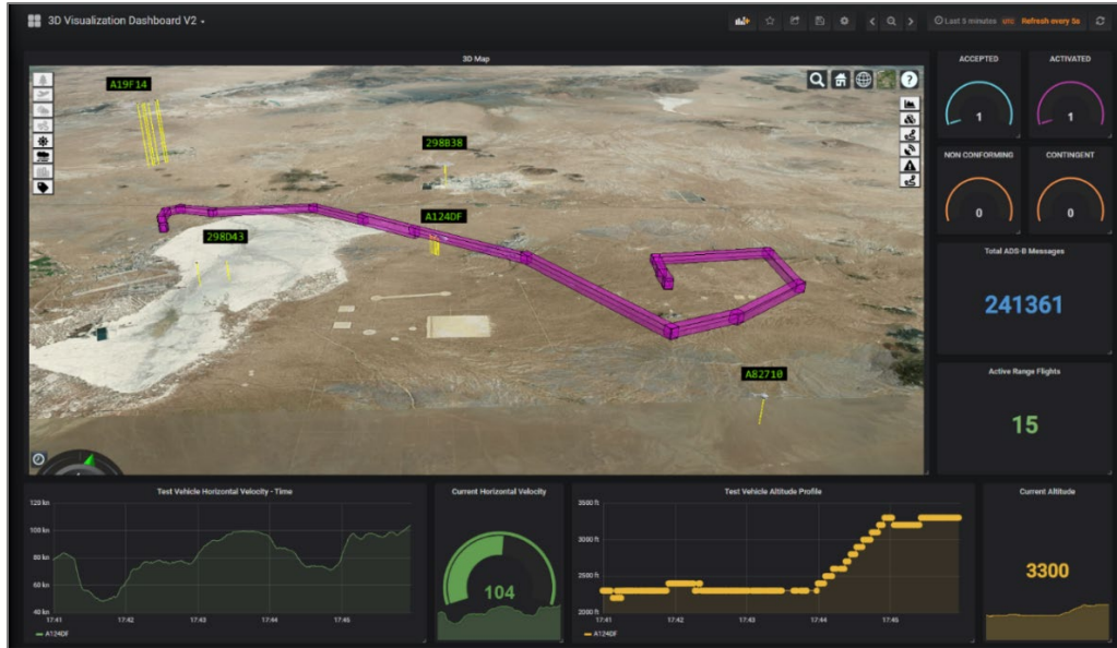
Figure 2.33. Grafana 3D Visualization Display for Real-Time Tracking.
