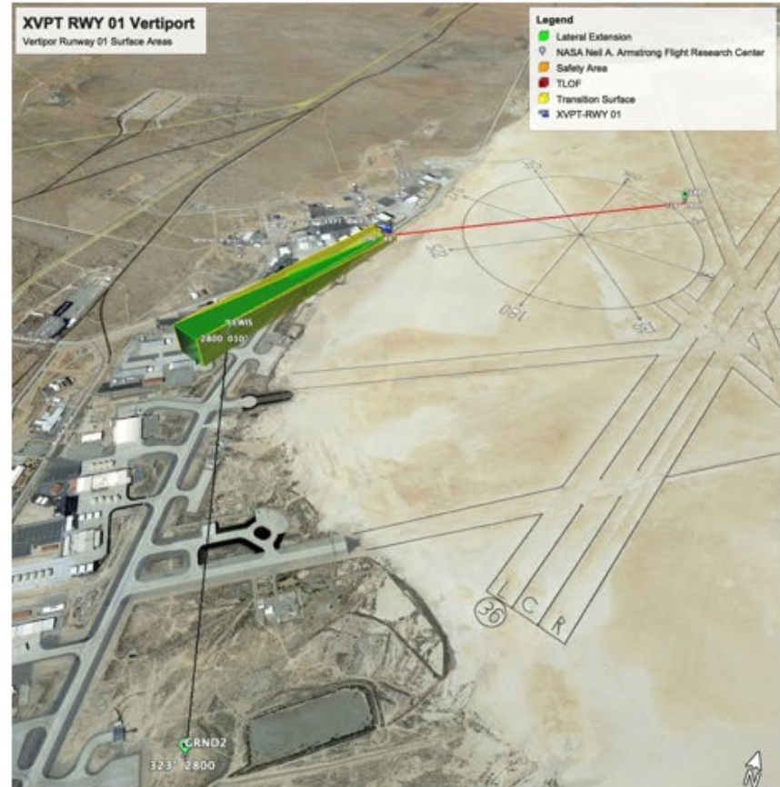
Depicts XVPT RWY 01 selected for short take-off and landing (stol) testing. the calculated magnetic variation, publication date, lat/long geodetic datum, and ellipsoidal heights in feet, surveyed thresholds required by the FAA to be accurate in any landing surface with a takeoff or approach procedure.
