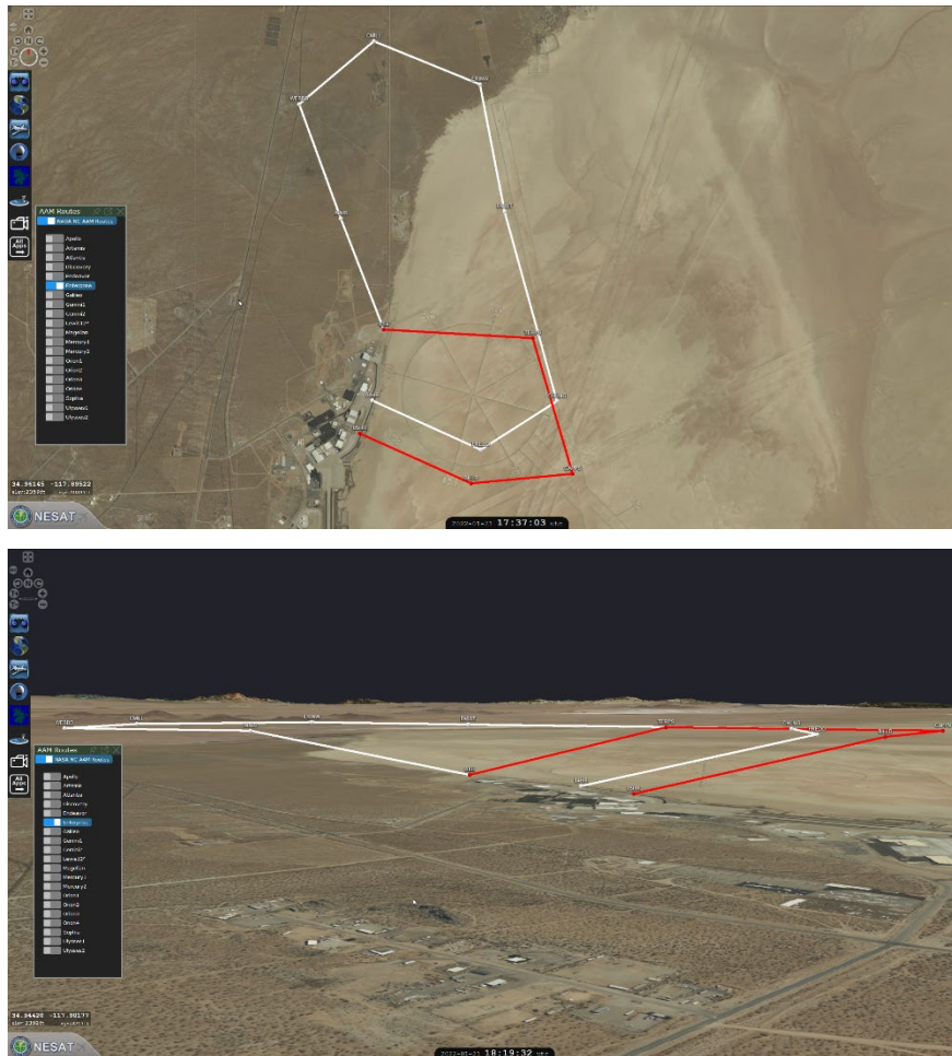
Figure 4.58. ENTERPRISE Balked Landing In SBSM (left); and as flown ADS-B track in Google Earth (right).
