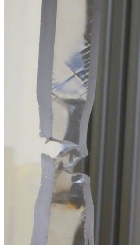
Typical Polycarbonate Break
