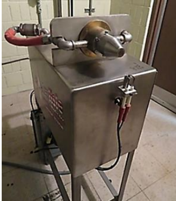
Figure 2: NG/O 2 burner rig and platform.
