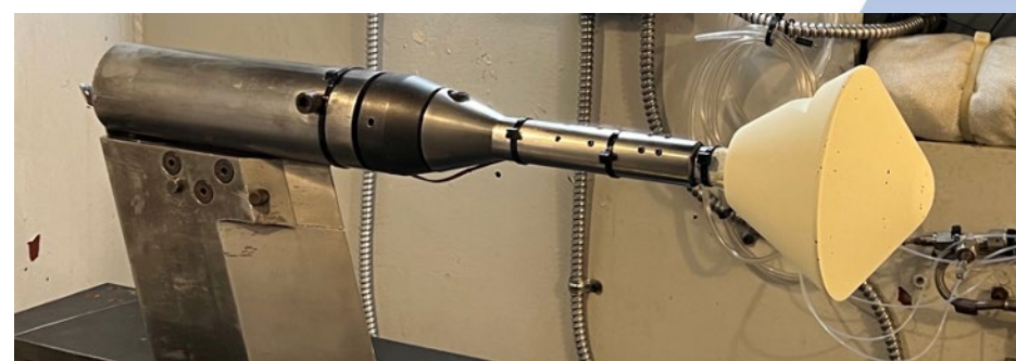
Mounted model in injection box of tunnel
