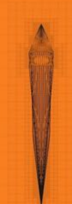
LAVA SR03 Stiff Radials + Viscous Log of density on surfaces and cut plane, where yellow is high and purple low, mesh shown in black
