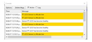
Example, of an inconsistency of a sensor, and this inconsistency is triggered by NPAS models being applied; physics, or other models in NPAS are detecting events; these events are used in root cause trees for diagnosis (as shown in example below)
