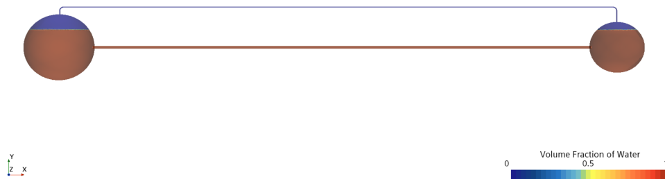
Figure 5: Initial CFD state of about 80% liquid fill.
