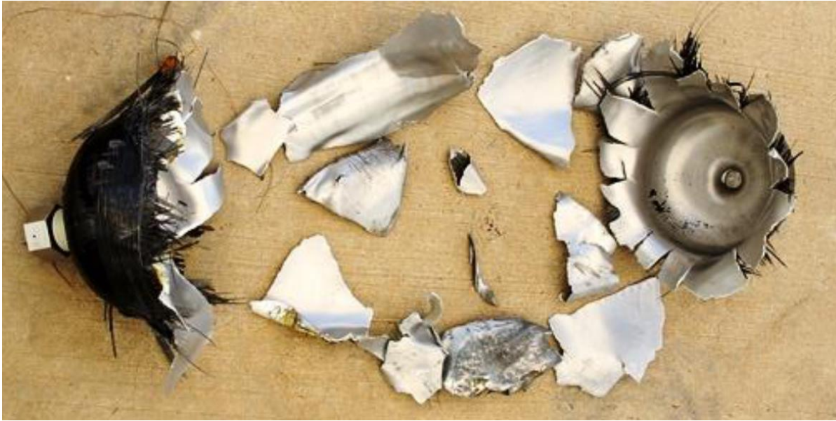
Figure 2. Example of a Ruptured COPV
