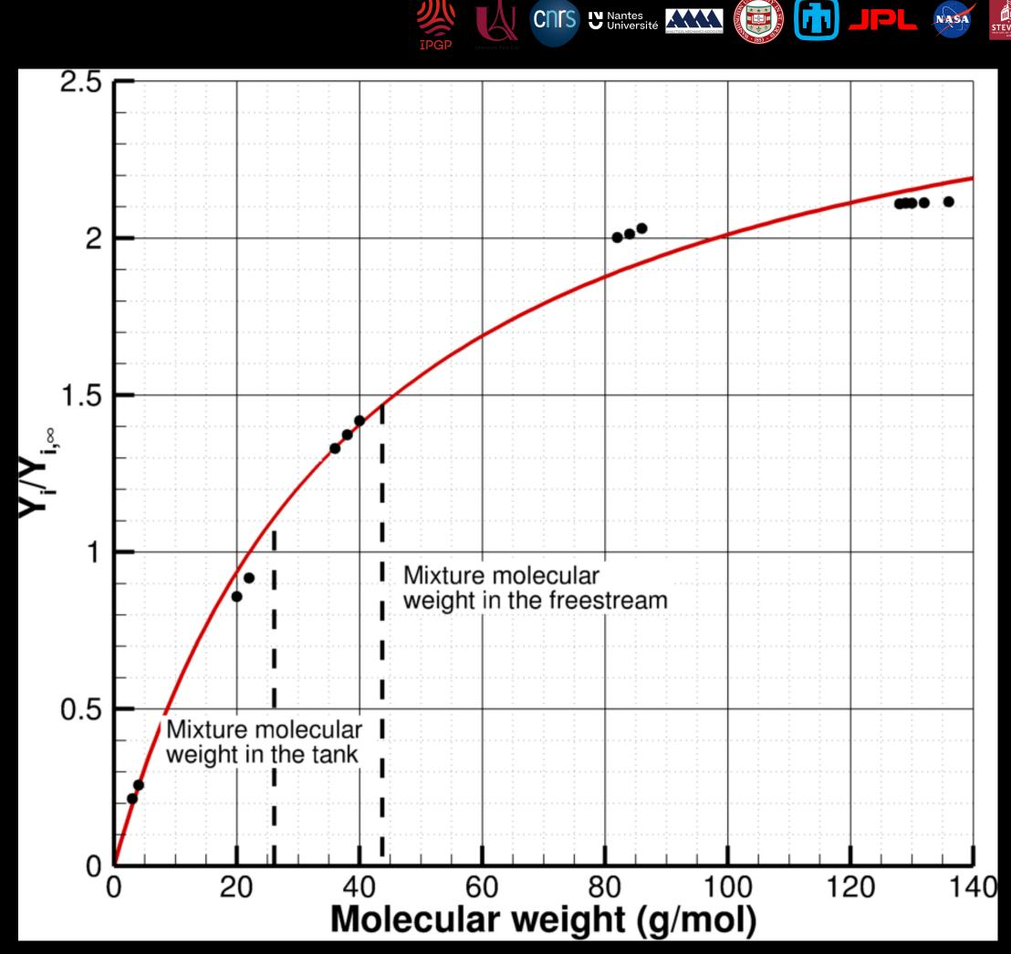
Fractionation is primarily driven by differential diffusion of species through strong bow shock, which itself is driven by molecular diffusion, and is a function of species molecular weight. Similar differential diffusion is observed for similar molecular weight species.
