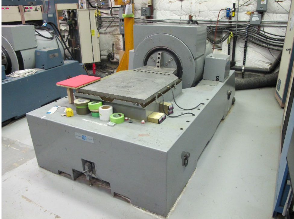
Figure 7. A Shaker table used for vibration testing at NASA AFRC.
