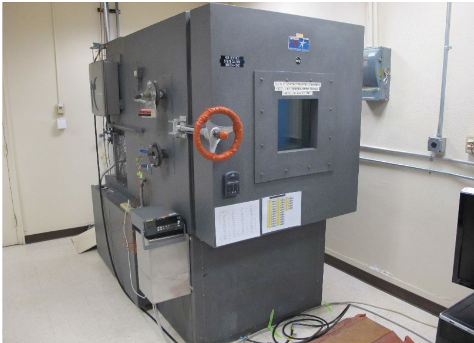
Figure 8. A Thermal chamber used for temperature testing at NASA AFRC.
