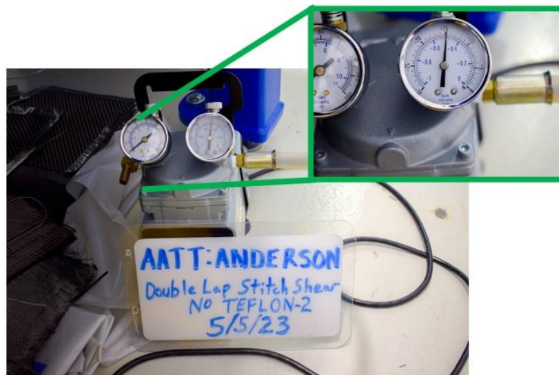
Figure A.5. Example vacuum pump gauge reading.
