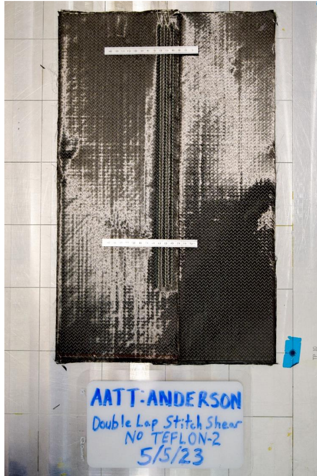
Figure 10. A completed dry specimen stitched under temporary vacuum consolidation after removal from vacuum bag.
