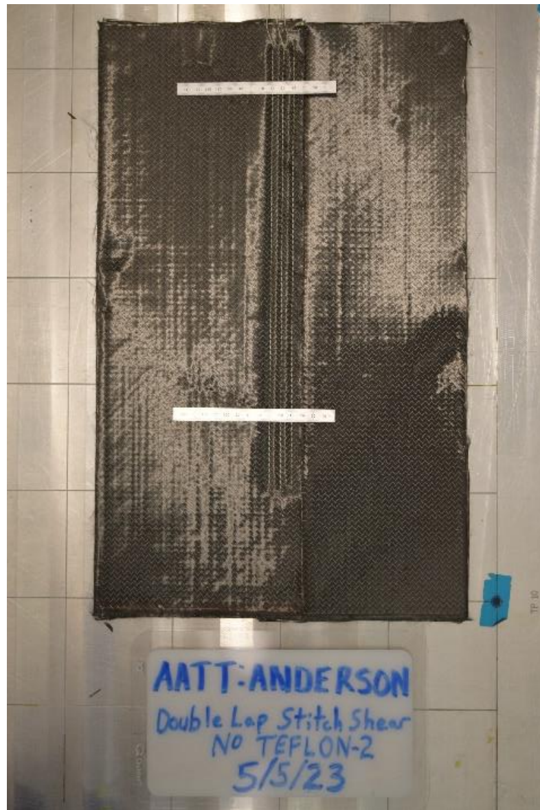
Figure A.10. Completed stitched preform.
