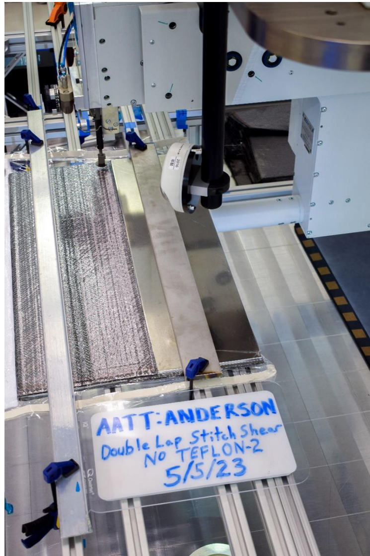
Figure 9. A temporarily vacuum consolidated preform being stitched.
