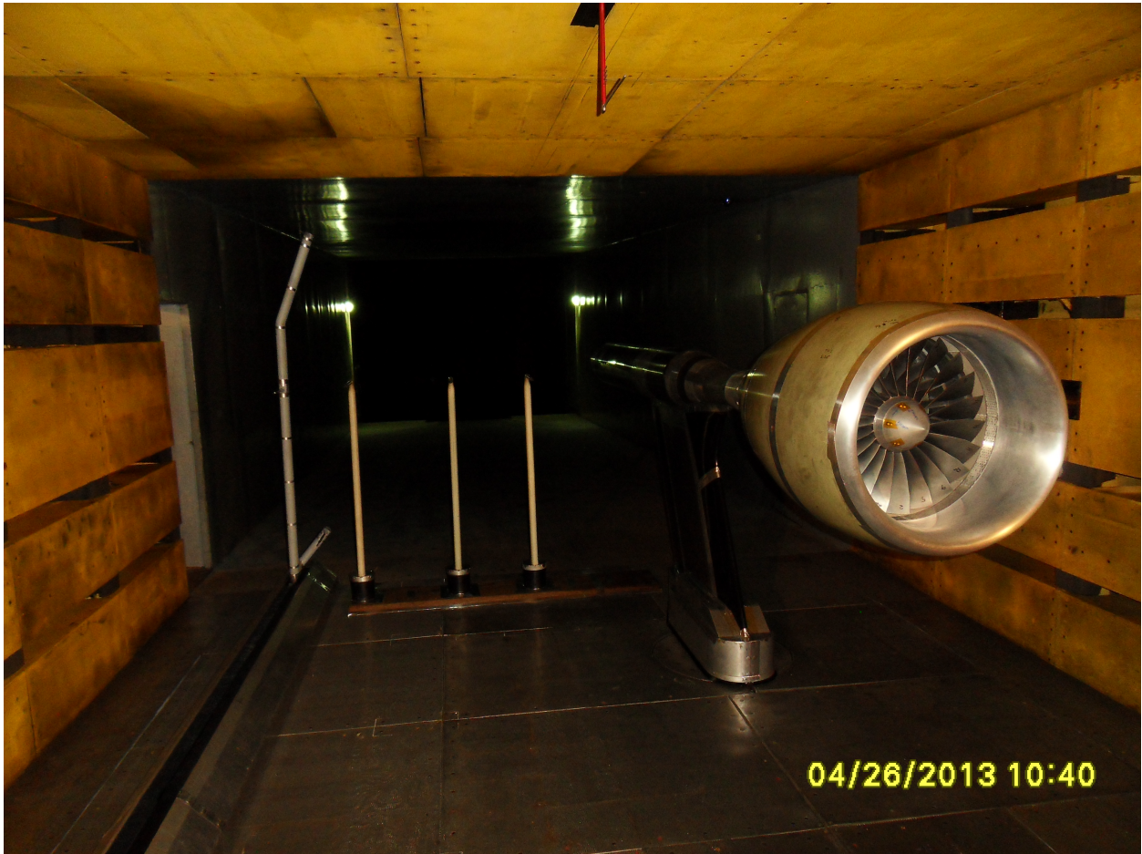
Figure 4.—Installed model in the NASA Glenn Research Center 9- by 15-Foot Low-Speed Wind Tunnel (9x15 LSWT) showing traversing and fixed microphone locations.
