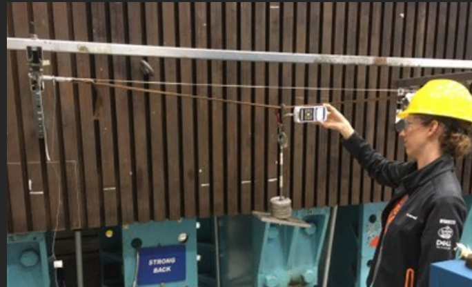
Test Conductor – Loads and pulls weighted carabiner and gets reading
