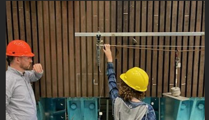
Secondary Test Conductor – The test process is easier and more accurate when a third person is present to aid in setup and to read off the scale
