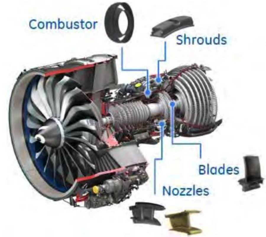
Figure 1. CMC components in an advanced GE jet aircraft engine. 2
