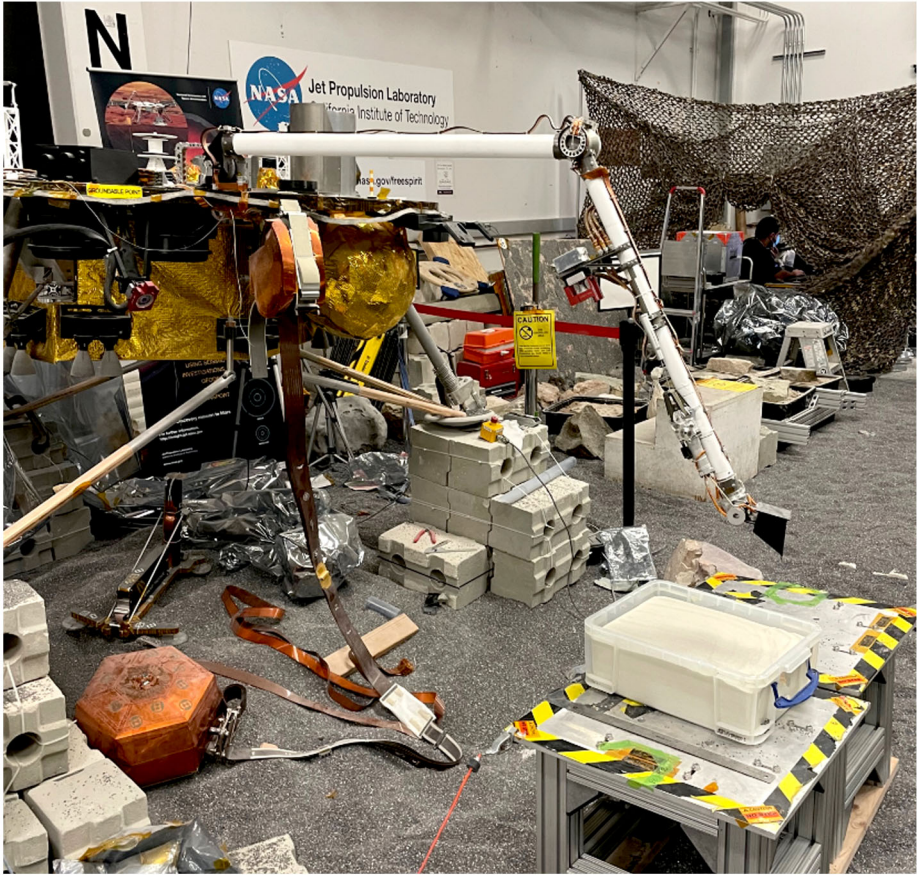
Fig. 27 Picture of the engineering model lander, robotic arm, and scoop in the JPL testbed. Note the container of simulant below the arm as well as the SEIS and HP 3 models on the surface to the left. The IDC is on the forearm of the IDA and the ICC is mounted beneath the deck to the left (with red around the lens). Note the lander feet were placed on cinder blocks to enable end to end testing of arm activities that assisted the HP 3 mole and interacted with the surface
