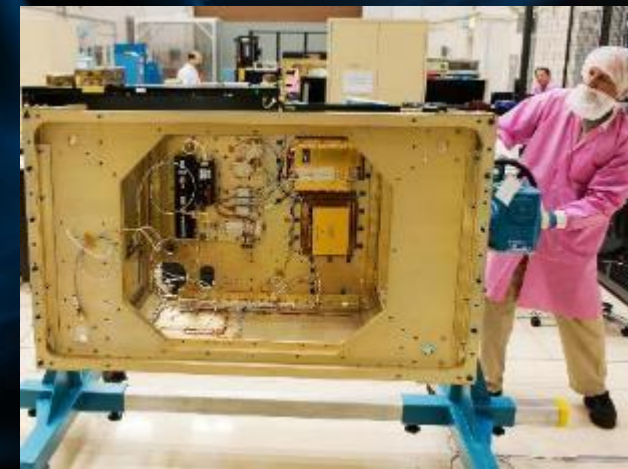
SCaN Testbed onboard the ISS to conduct software defined radio (SDR) experiments
