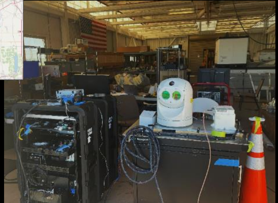
Laser Ground Terminal near GRC hangar
