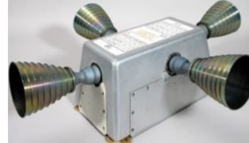
Apollo CSM RCS using C103. Courtesy Aerojet-Rocketdyne
