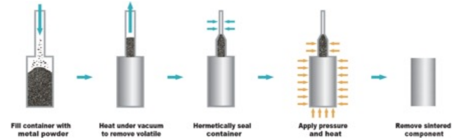
Hot Isostatic Press (HIP) process [1].
