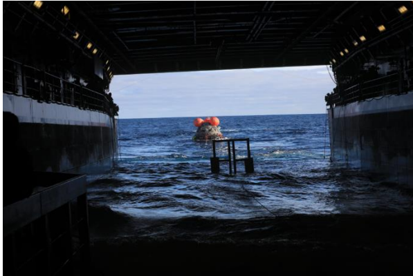
Fig. 11. Orion CM recovery into the well-deck of the USS Portland
