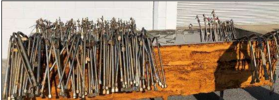
Figure 7: Photograph of the water tank and immersed test articles used for leak testing of CRES tubing test assemblies.
