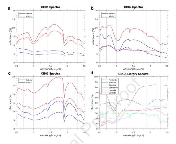
Figure 3 – VNIR spectra of the boninites. A) Sample CB01; B) Sample CB02; and C) Sample CB03. Representative spectra of both exteriors and cut interiors are plotted, demonstrating the approximate range in reflectances observed.
