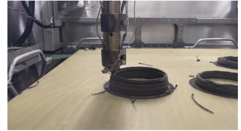
Samples were printed under vacuum ( 10^{-3} torr)
