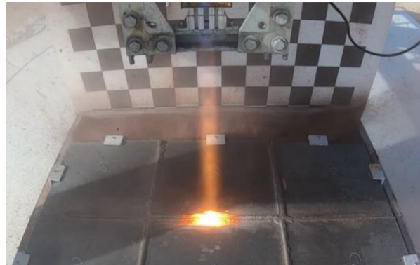
Paver grouting mitigates hot fire conditions
