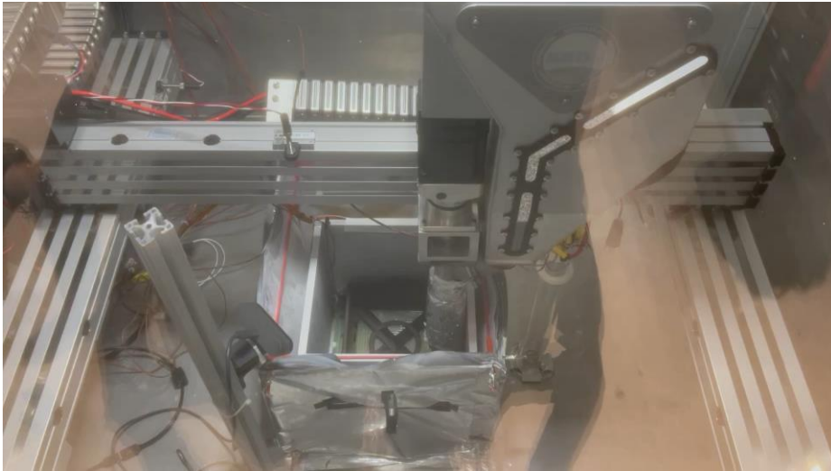
Test samples are printed in TVAC conditions
