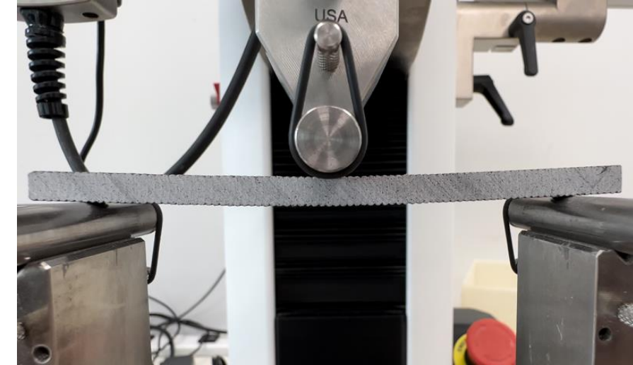
Formulations undergo flexural testing
