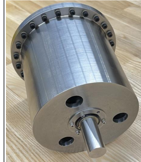
Assembled cycloidal magnetic gear (left) mounted for testing (right)
