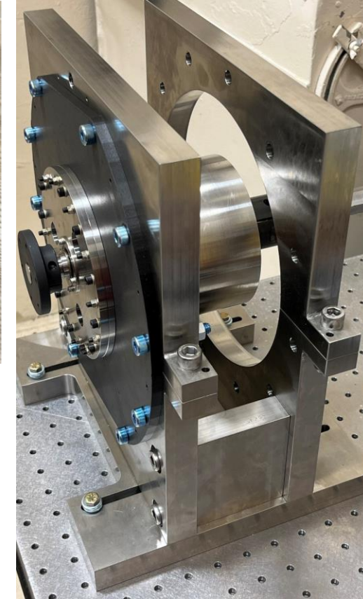
Assembled cycloidal magnetic gear (left) mounted for testing (right)
