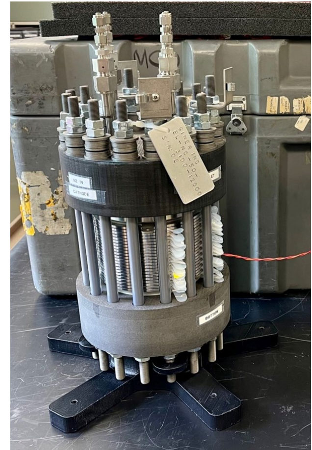
RFC project Liquid Anode Feed Water Electrolyzer manufactured by Giner on 3D printed support fixture at GRC
