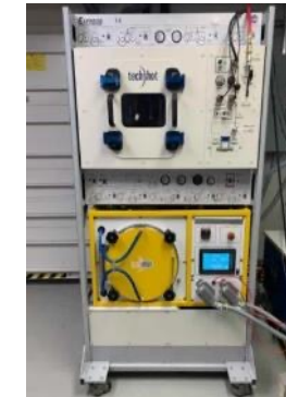
FabLab (multimaterial printer for \mu g application)
