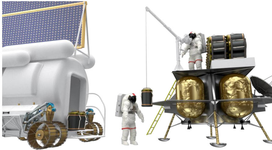
Figure 19. Concept depicting use of davit to offload 1.0 SPLCs to the airlock/Pressurized Rover.
