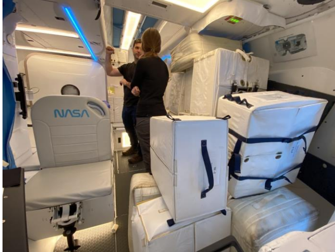
Figure 18. Habitable airlock mockup at JSC with 37.5 CTBE in soft bags; interior volume ~ 9.5 m 3 .
