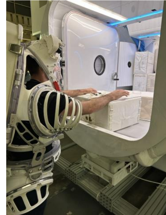
Logistics test at JSC mockup utilizing various CTBEs
