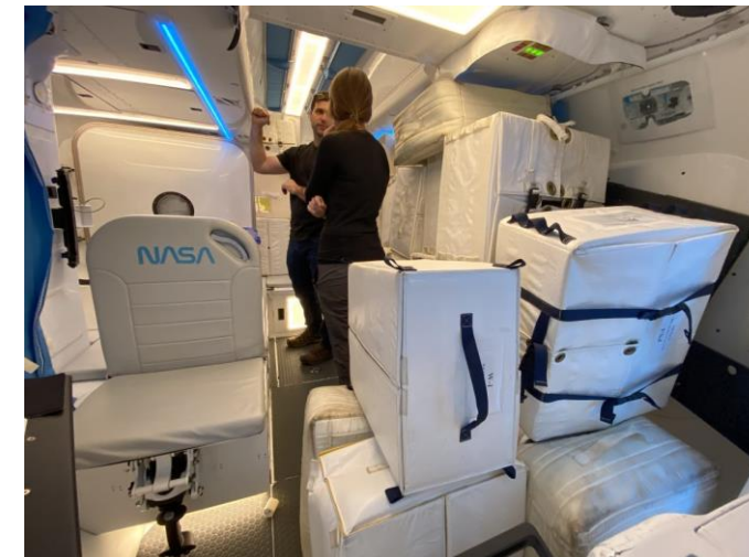
Habitable Airlock mockup at JSC with 37.5 CTBE in soft bags; interior volume \sim 9.5 \text{ m}^3
