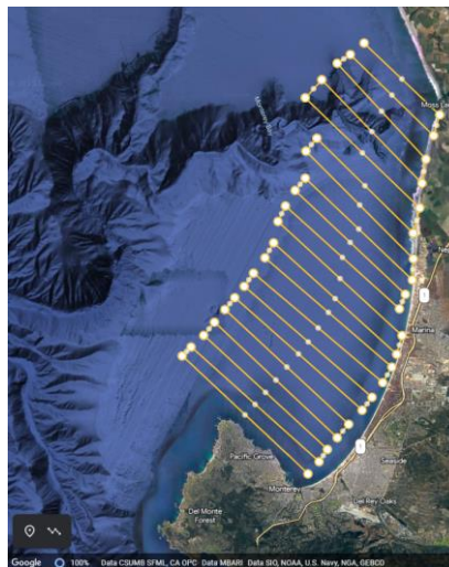
Fig. 6 Example pathing for a surveying drone covering half of Monterey Bay.
