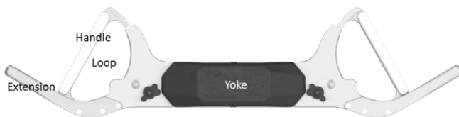
Figure 40. The physical elements of the Tri-Rotor controller [MSC-27385-1 under NASA patent review].
