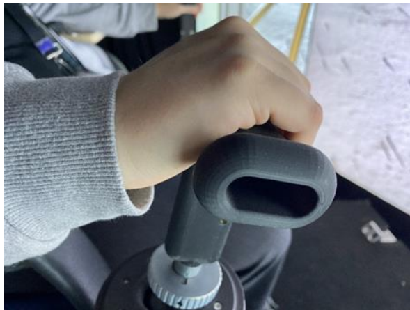
Figure 28. Gripping the LTV dual T-Handle controllers was considered easy and comfortable in rough terrain.
