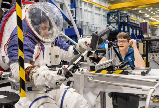
Figure 43. Pressurized suit subject testing the Tri-Rotor controller.
