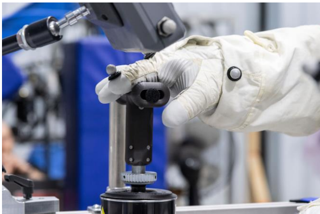
Figure 29. A 4.3 psia pressurized gloved hand gripping the LTV T-Handle controller.
