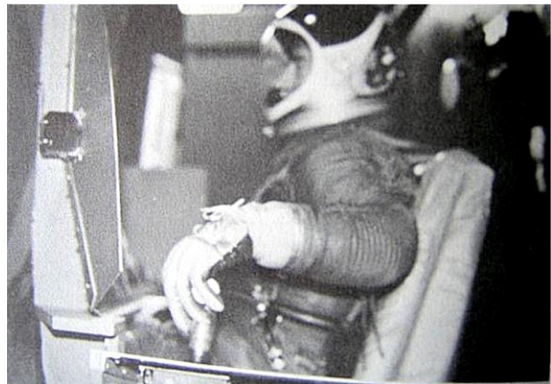
Figure 5. Astronaut John Young in a space suit driving the MSFC LRV Simulator using the T-Handle. [3]
