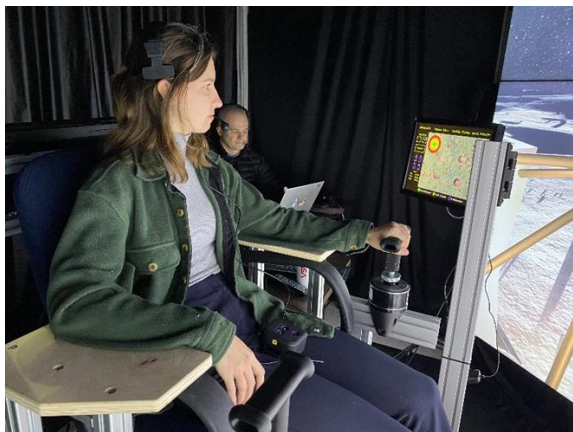
Figure 32. With cruise control activated, it was easy for a subject to drive single handed reducing fatigue.
