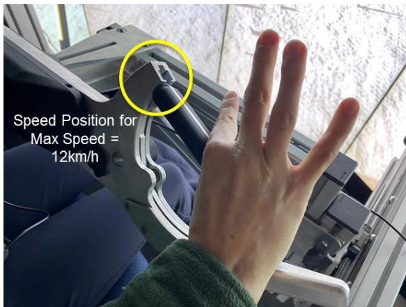
Figure 49. Subject pushed the speed loop all the way passes the handle frame to obtain max speed.
