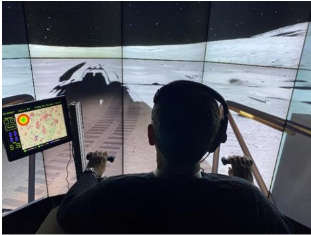
Figure 27. Reach to the LTV dual T-Handle controllers was considered comfortable.
