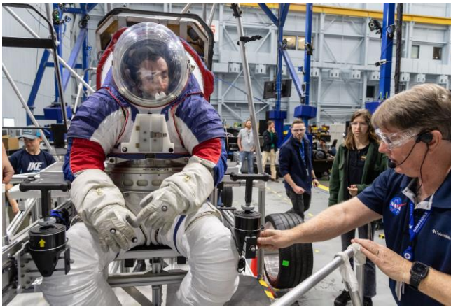
Figure 25. Test team working with subject in the side entry mockup vehicle.
