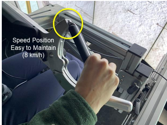
Figure 48. The speed loop flush to the handle frame was the position for maintain speed but not max speed of the vehicle.
