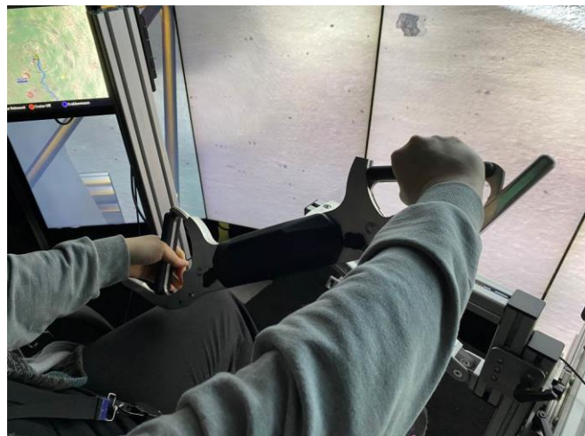
Figure 42. Note the Tri-Rotor controller hitting the subject's leg caused by a weak spring mechanism.
