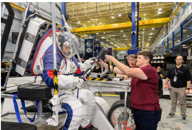
Figure 26. Test team working with subject in the front entry mockup vehicle.
