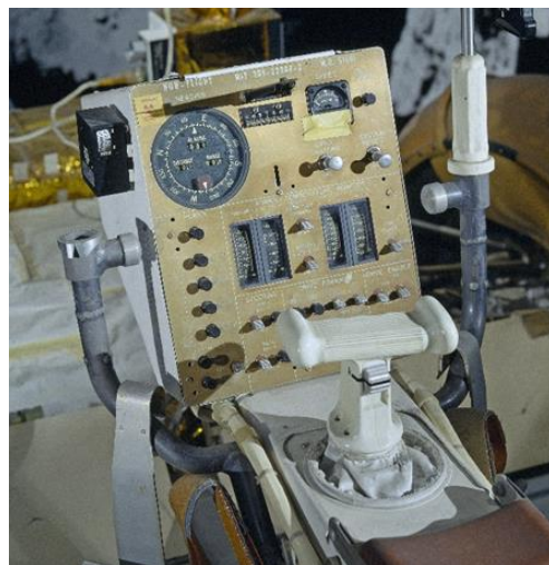
Figure 6. The Apollo LRV T-Handle controller and center display panel. [Curiosity NASA]
