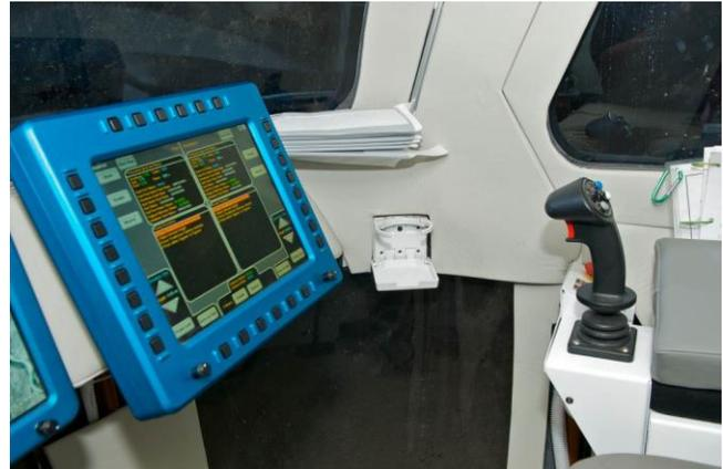
Figure 15. The CH Product MV4 Joystick in the SPR Generation 1B cockpit during field testing in 2009.
