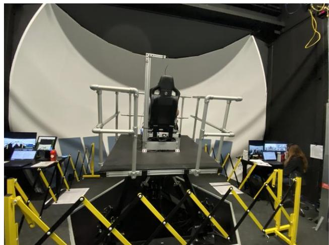
Figure 16. The motion table in the SES Mini Dome facility.
