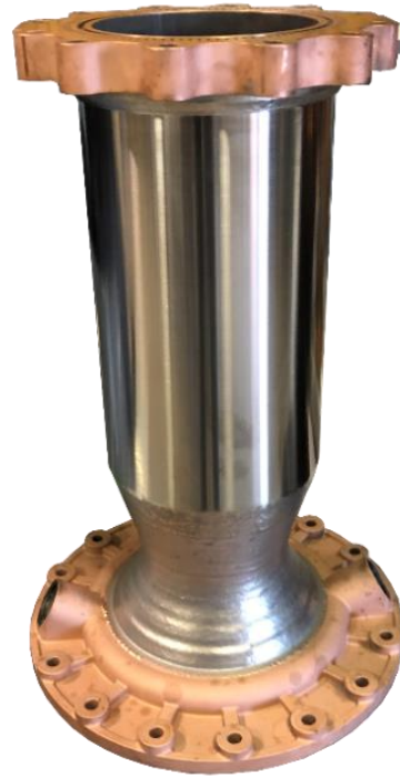
L-PBF Liner / Coldspray Jacket
