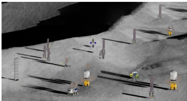
Fig. 3. Concept of distributed power sources with associated loads during lunar south pole operations
