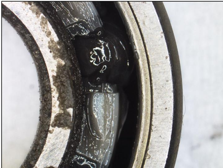
Photograph of damage (denting) on inner raceway
