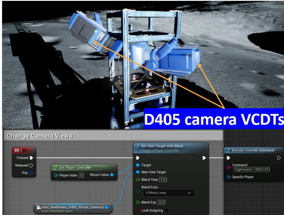
Fig. 17 Synthetic image dataset collection blueprint with depiction of multiple game assets for switching between D405 camera VCDT camera angles
