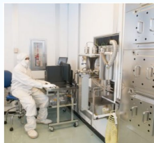
Oxidation and Annealing Furnaces and Silicon Dioxide Low Pressure Chemical Vapor Deposition System
