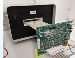
Insertion of SiC Chip on Ceramic Board Into Oven
