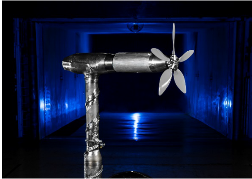
Tilting Proprotor (14'x22') Aero Performance - VFS 79-2023-0140 Acoustic Test – 2025
