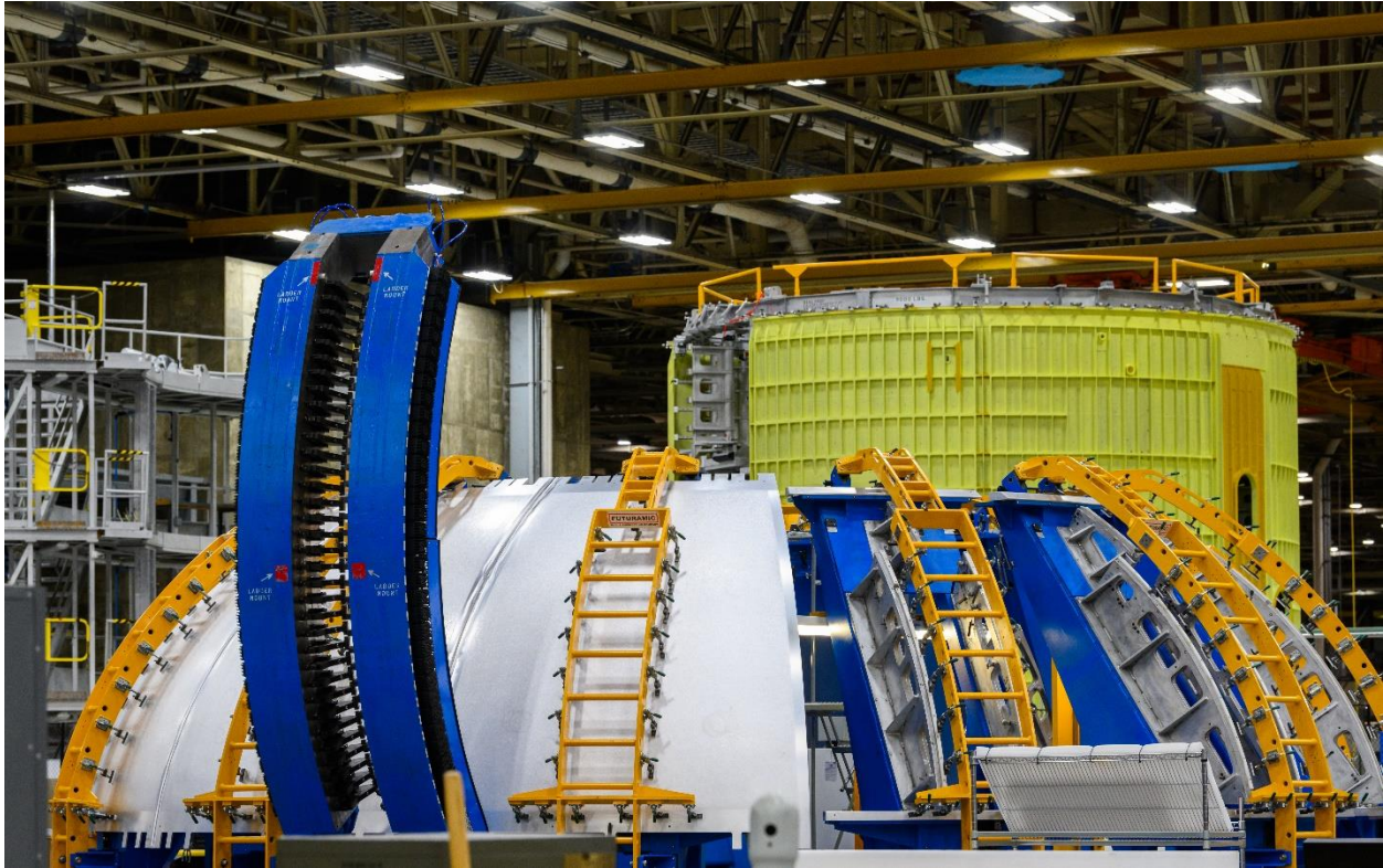
Fig. 7 The Artemis IV LOX dome, forward, and intertank, background, are being manufactured at Michoud. Shown are weld confidence articles.
