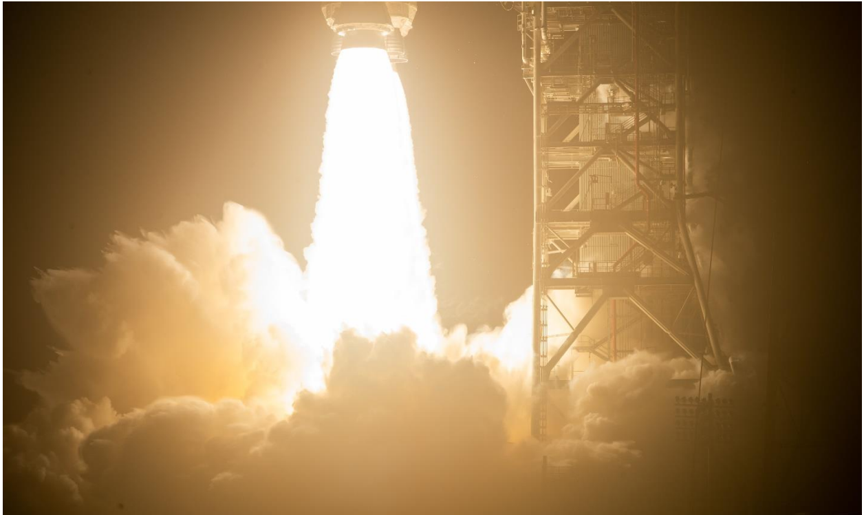
Fig. 4 The Artemis I SLS's twin solid rocket boosters and four RS-25 engines propel the rocket and spacecraft off the launch pad for the first time on Nov. 16, 2022.
