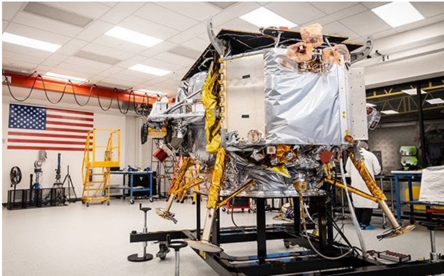
(Left and center) OPAL camera (red lens cover) shown fully integrated on Peregrine lunar lander prior to environmental acceptance test campaign. (Right) OPAL Systems Engineer Holly Lindenfelser participating in Peregrine lander mission simulations.
