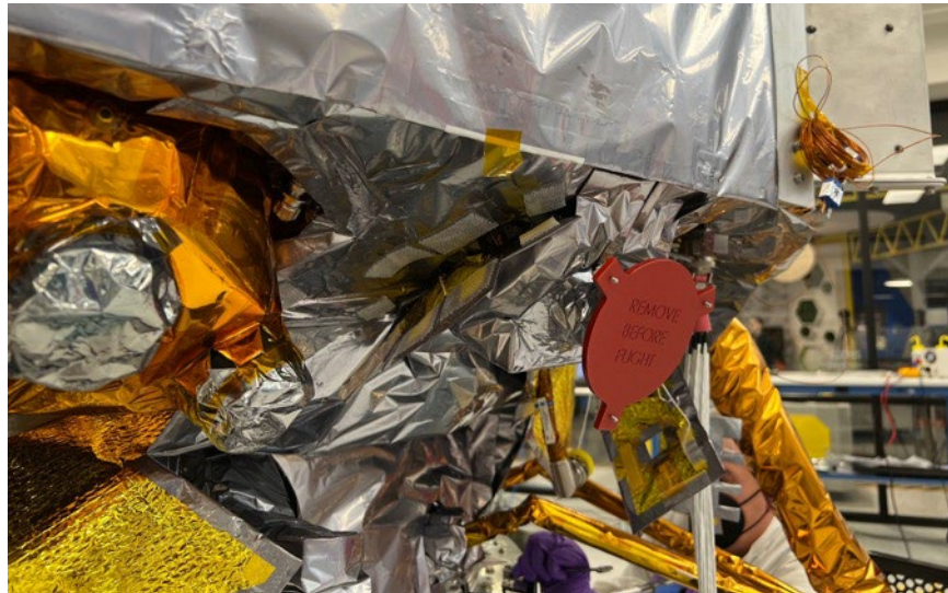
(Left and center) OPAL camera (red lens cover) shown fully integrated on Peregrine lunar lander prior to environmental acceptance test campaign. (Right) OPAL Systems Engineer Holly Lindenfelser participating in Peregrine lander mission simulations.
