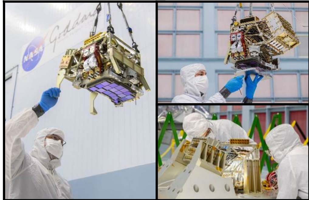
Focal Plane Assembly (FPA) after successful vibration testing. FPS assembly and thermal vacuum testing complete. FPS shipped to Ball in early May
