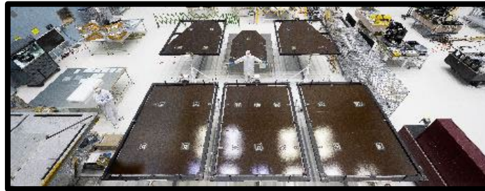
Spacecraft Solar Array Sun Shield (SASS) panels – 6 flight SASS substrate panels shipped to cell vendor in March for cell laydown
