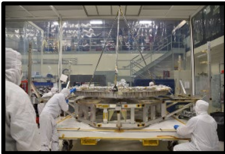
Prop Deck Subassembly Lift to Prop Support Frame in B11 High Bay
