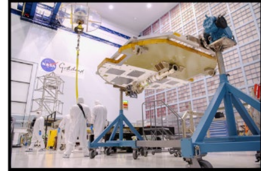
Spacecraft High Gain Antenna System (HGAS) – assembly underway in SSDIF
