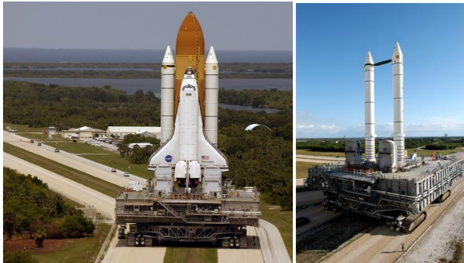
Figure 10. Shuttle-Era CT transporting Space Shuttle on the MLP (left), Partial Stack Rollout (right)
